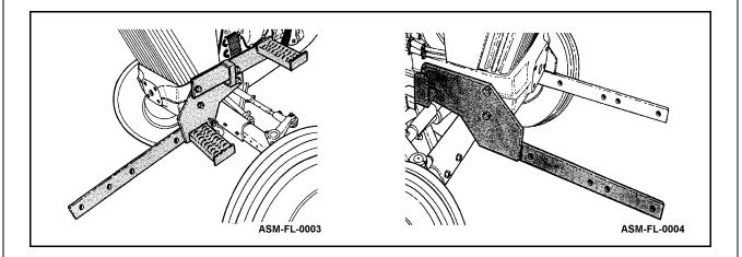
Position the mainframe under the tractor. Lift the front of the frame and install the top two 5/8" x 2" bolts. Install a 5/8" flatwasher and a 5/8" locknut on the bolts and tighten enough to hold the frame in place. ASM-FL-0005
